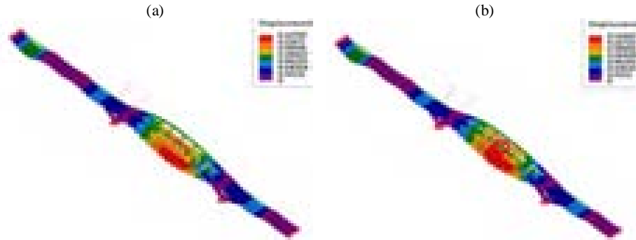
Fig. 4. Bridge displacements: (a) dead weight, (b) dead weight and static wind action.
