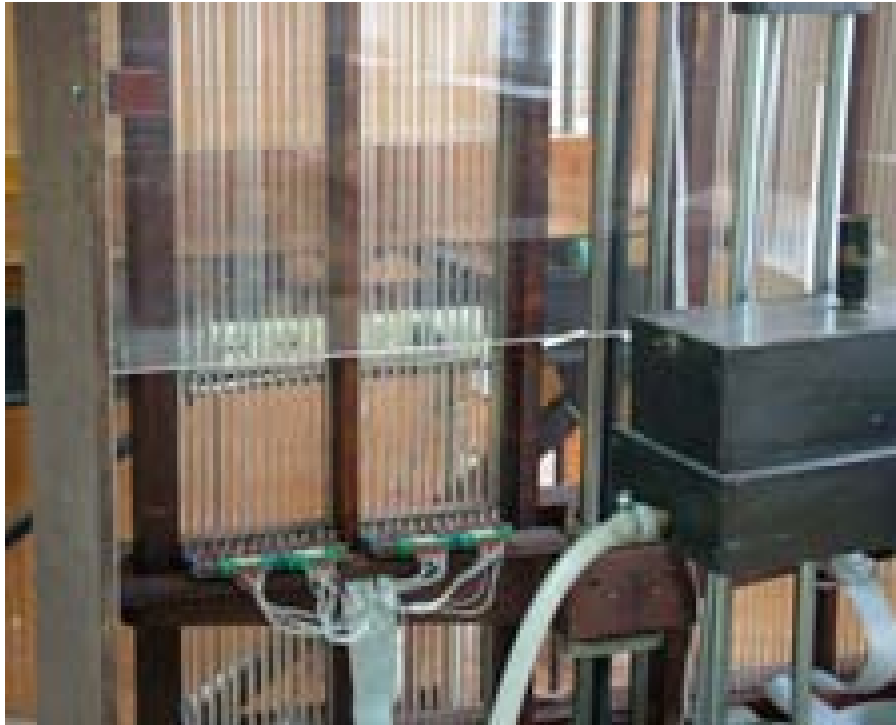
Fig. 3. Multipunctual liquid manometer.
