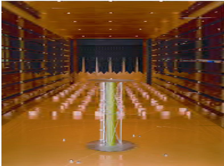
Fig. 4. Sectional model of a steel chimney in a frame-truss housing.
