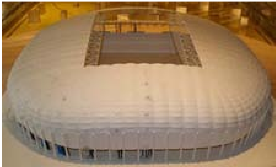
Fig. 12. Wind tunnel tests of stadium roof in Poznań.
