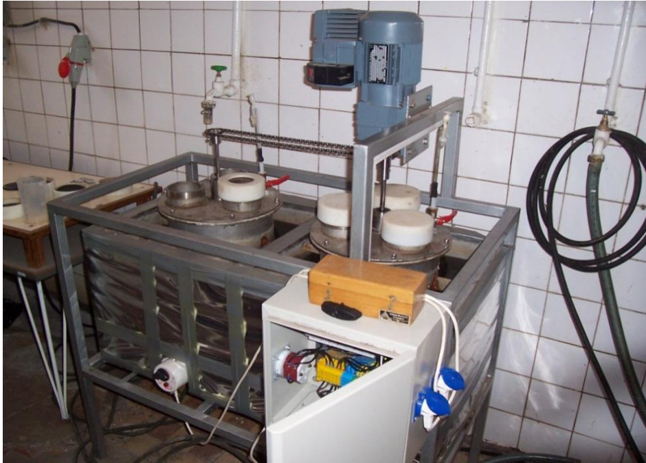
Fig. 2. 2 bioreactors thermostatic in water bath
