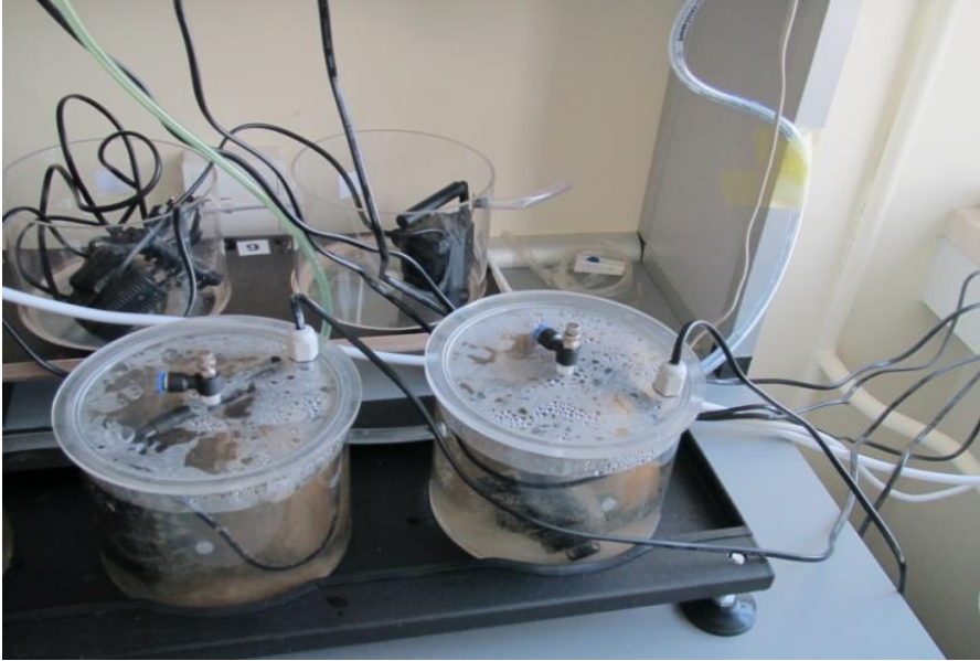
Fig. 1. Photo of an experimental model of a two-stage anaerobic bioreactor with microorganisms immobilized on carriers
