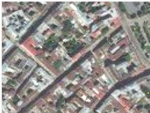
Fig. 9. Fragment of a satellite image of the city of Lviv with examples of determining the types of coverage: blue (dark) cells – impervious surfaces; yellow (light) cells – water-pervious surfaces
