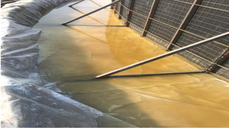
Fig. 2. Filtration of water through the wall of the installation, after treatment of drilling waste with flocculants
