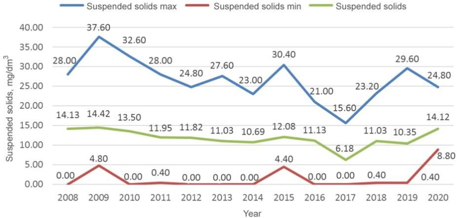
Fig. 10. Changes in the suspended solids
