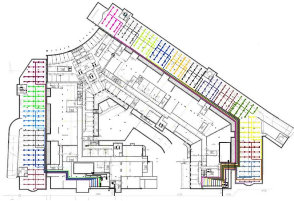
Fig. 3. Proposed Variant IV, nozzles installation
