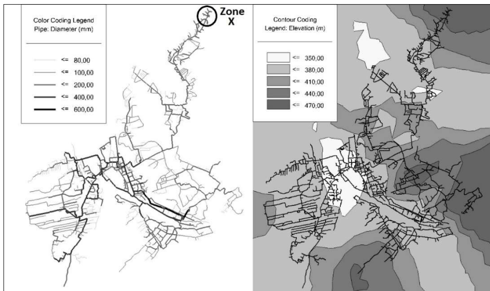
Fig. 1. Geometrical structure of the WDS with pipe diameters and elevation contours and marked zone X
