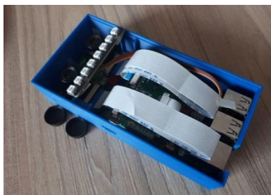
Fig. 4. Device for stereoscopic images of skin lesions
