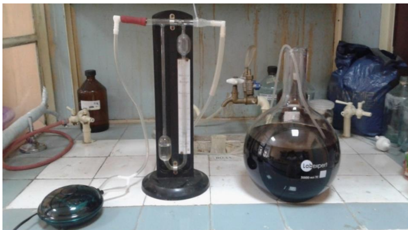
Fig. 2. Experimental lab-scale installation for the study of aerobic leachate pretreatment
