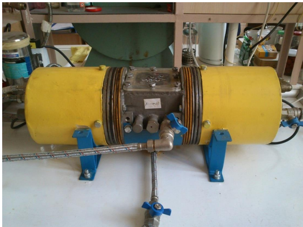
Fig. 1. A picture of a low-frequency vibratory resonance cavitator for cavitation treatment of aqueous solutions with a high content of MPN_0 and COD under pressure and at high temperatures
