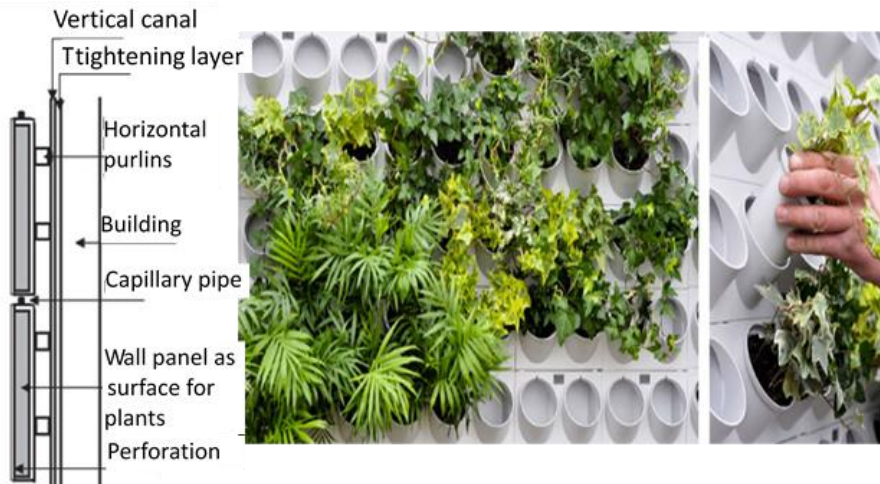
Fig.6. Module method used for vertical garden creation (Furmanik 2010; http://gardenspot.pl )
