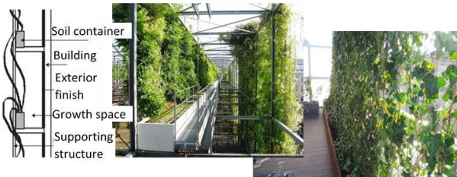
Fig.7. Container system used for vertical garden creation (Furmanik 2010; http://blog.gcl.com.pl , http://www.gabiony.poznan.pl )
