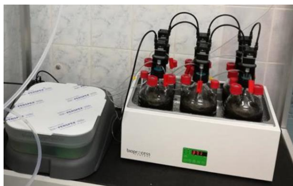
Fig. 1. BioReactor Simulator (BRS): anaerobic reactors (BRS-A, unit in the right), gas volume measuring device (BRS-B, unit in the left)
