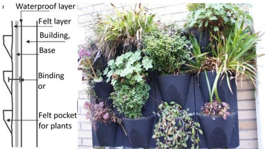
Fig.4. Felt method used for vertical garden creation. ( https://architekturakrajobrazublog.wordpress.com )
