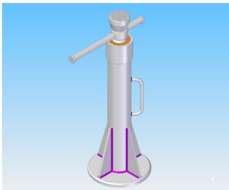
Pic. 1.2. Screw lift with drive through the screw – 3D model
