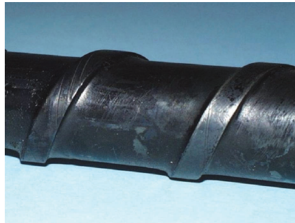
Fig. 16. Appearance of the screw applied to SAN processing that shows the abrasive wear in the feeding zone
