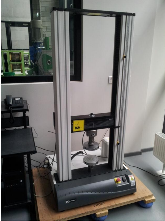
Fig. 2. Test stand: a) Machine Instron 3369, b) Manual jaws Instron 50 kN, c) 3D printer uPrint SE [source: own research]
