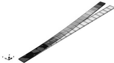
Fig. 7. The bending natural mode shapes of the beam in the rigid direction (plane: x_2 - x_1 )
