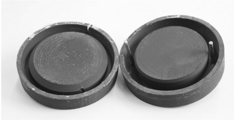
Fig. 4. Halves of the casting mold produced using FDM technology [source: own study]
