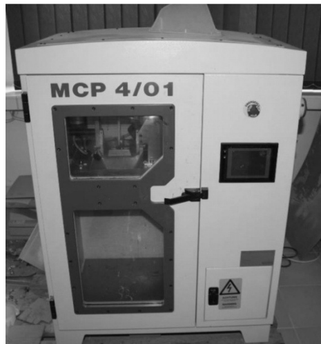
Fig. 6. Vacuum chamber MCP 4/01 used for silicone degassing [source: own study]
