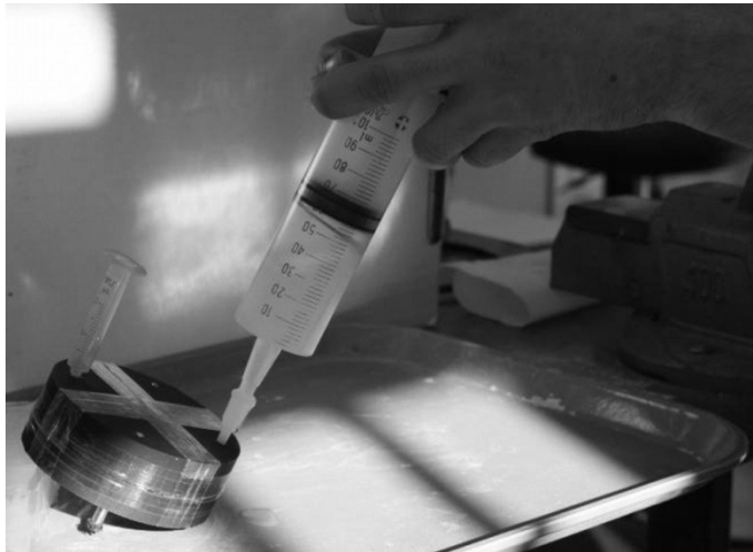
Fig. 7. Pouring the silicone into the mould [source: own study]
