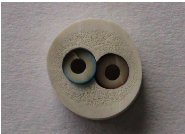
Fig. 7. Structure view of PVC double-layer cable, magnify 20x
