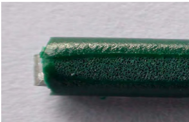
Fig. 5. View of bended double – layer wire with 32% degree of porosity
