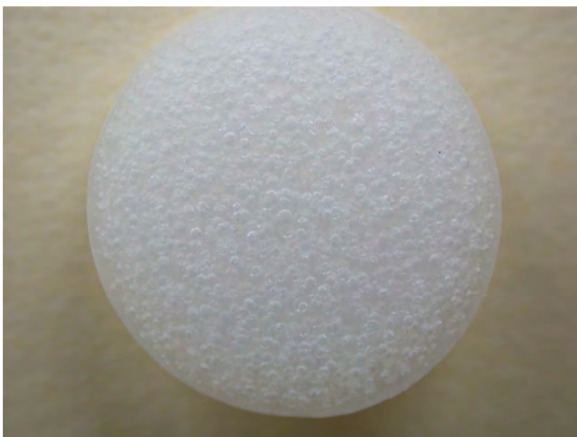
Fig. 3. Cross – section view of PE-HD cellular singlelayer
