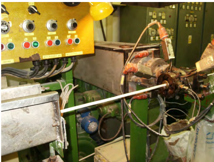
Fig. 6. Fragment of cellular co-extrusion line of PVC cable layer
