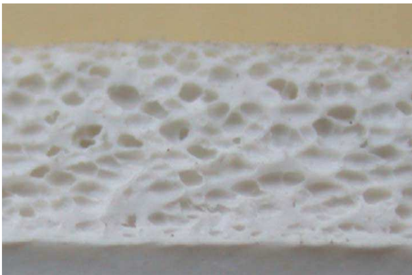
Fig. 2. Microscopic image of the cross section of the cable covering made of cellular polymer of the amount of the endothermic blowing agent 0.6% mass.
