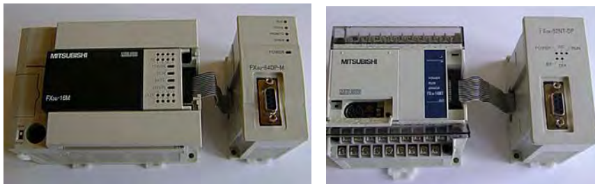
Fig. 4. Mitsubishi PLC controllers with Profibus DP modules: a) FX3U-16MT/DSS with an FX3U-64DP-M module, b) FX1N-14MT/DSS with an FX0N-32NT-DP [10]
