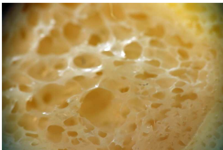
Fig. 9. Microscopic image of the cross section of the cable coating made of cellular PVC of the amount of the blowing agent (PLC 751) 1,0% mas., magnify 100x
