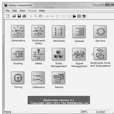
Fig. 5.2. SimEvents block libraries for building discrete-event simulations
