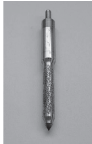
Fig. 4. Needle with the catalytic coating applied on the non-working part [8]
