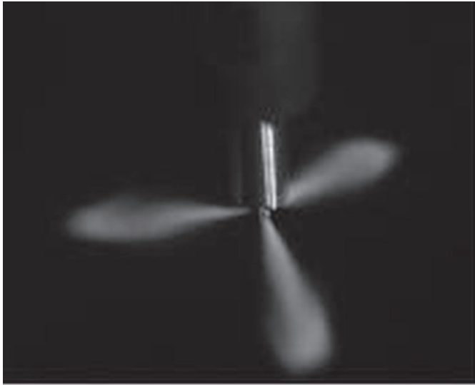
Fig. 5. Stream of the fuel injected in the factory injector
