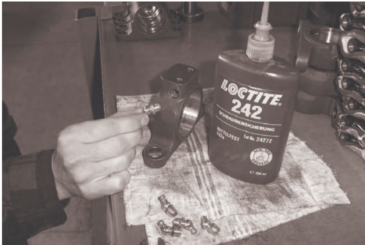
Fig. 2. A lubricating nipple secured with an anaerobic threadlocking agent
