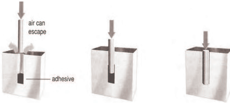
Fig. 6. If a blind drilled hole is used as an "adhesive reservoir", the adhesive is generally prevented from being pressed out by compressed air when the parts are joined. Adhesive waste can be minimized in large parts with the use of rubber plugs in the holes. In the case of blind holes, applying adhesive to the stud will result in lower than desired strength due to lack of adhesive getting into the joint [10]
