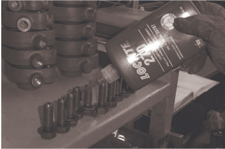
Fig. 1. Example of using glue to protect screws in power transmission system
