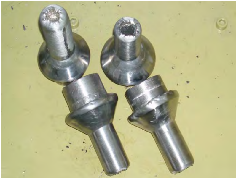
Fig. 5.4. Full and hollowed products obtained in rolling extrusion process (material – commercially pure lead)
