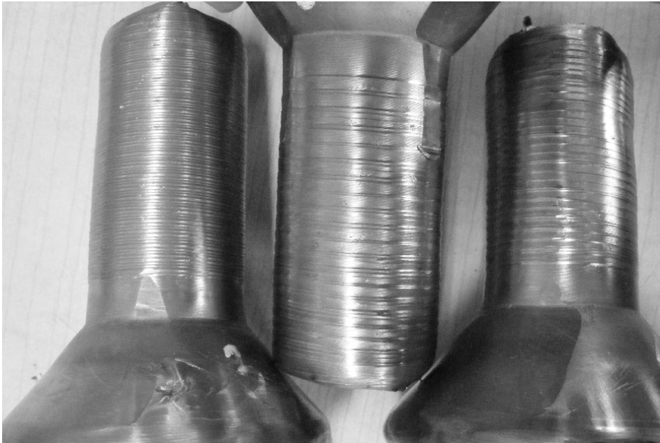
Fig. 5.1. Rotary extruded products made from lead Pb1 during functional – movement tests of aggregate PO – 1 without the application of rotary head mounted on pusher
