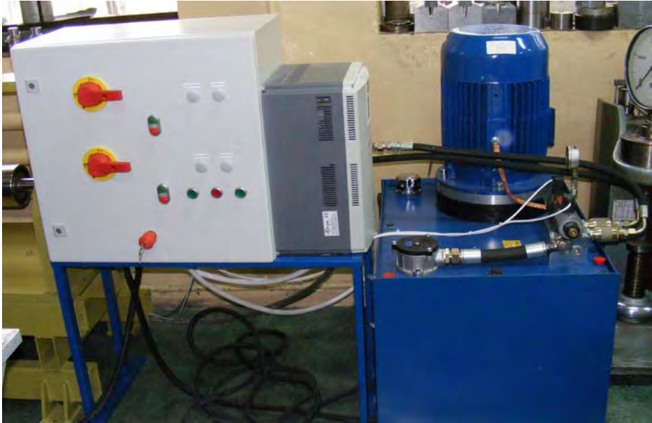
Fig. 4.5 .Steering unit with steering panel and vector inverter and hydraulic servo-motor equipped with steering valves
