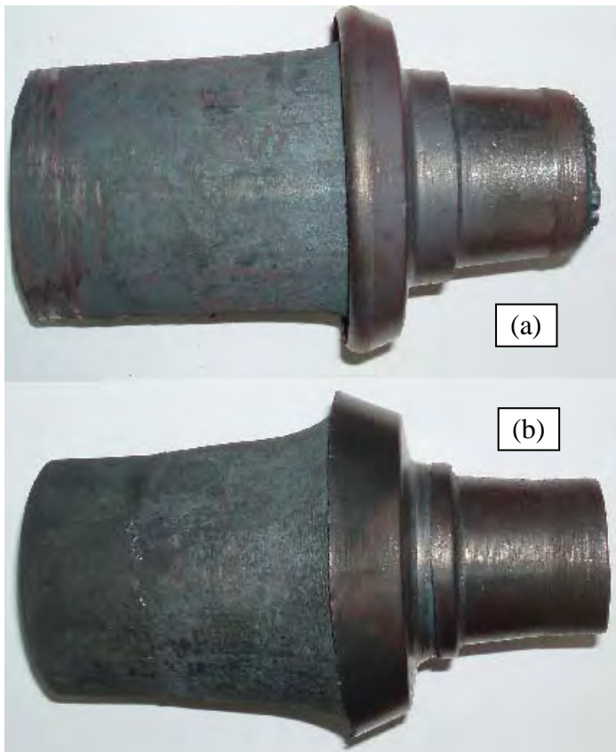
Fig. 6.6. Influence of various values of feed on rotation p on finished product obtained shape: (a) p = 2,5 mm/rot.; (b) p = 7,5 mm/rot.
