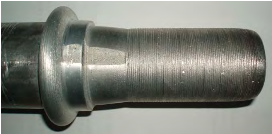
Fig. 6.7. Marking of tools rolls outline on rotary extruded full product ( p = 7.5 mm/rot.)
