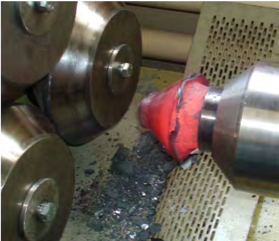
Fig. 5.12. Phenomenon of excessive billet upsetting before tools rolls forming zone ( p=1 mm/rot.)
