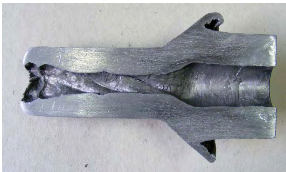
Fig. 5.6. Longitudinal section of hollowed product made from commercially pure lead after rolling extrusion process ( p=5 mm/rot.)
