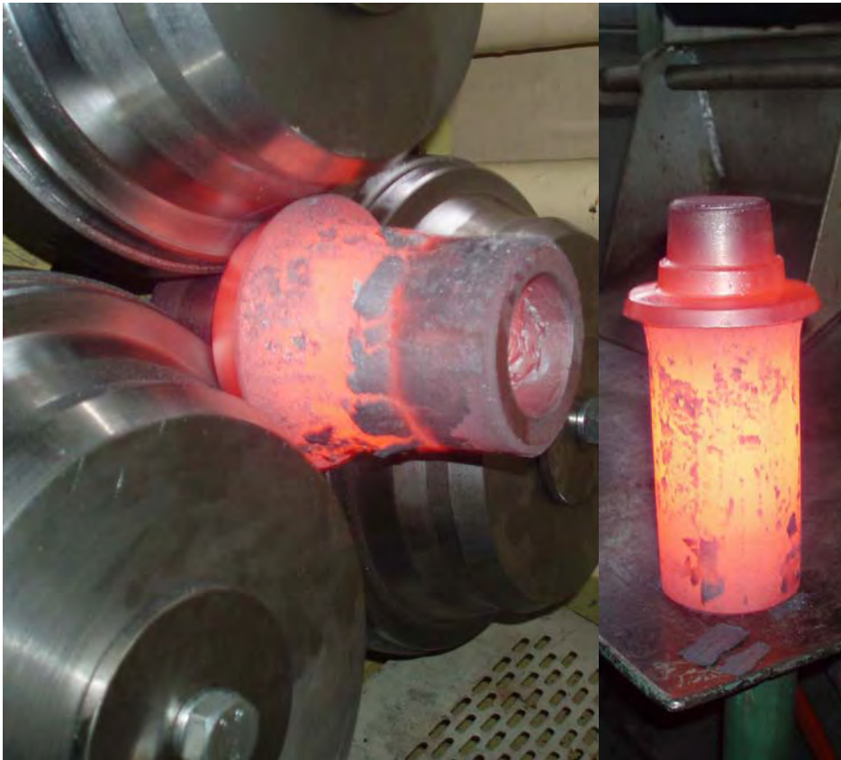
Fig. 6.5. Rolling extrusion process of stepped hollowed shaft with the application of designed rolls tools and obtained full product ( p=5\text{mm/rot.} )
