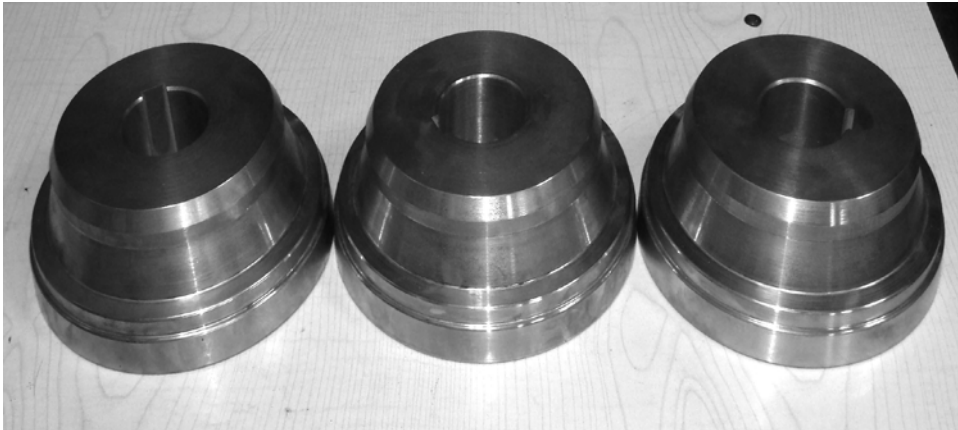
Fig.6.4 Working rolls for rolling extrusion process made according to Fig. 6.2
