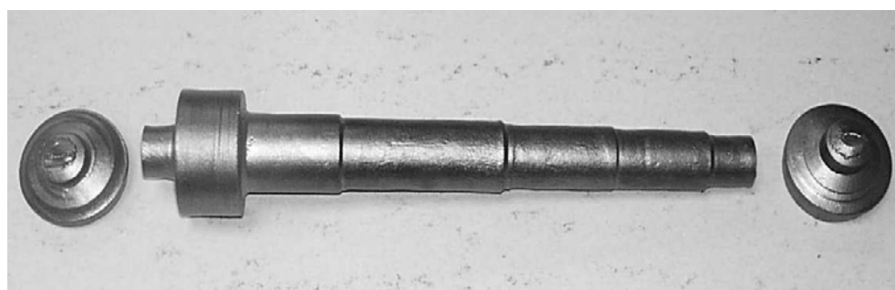
Fig. 2.23. Forging of mean shaft together with final waste cut during CWR process [40]
