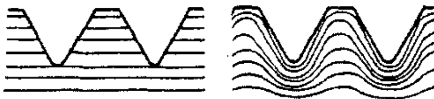
Fig. 2.5. Material fibres distribution after machining (at the left) and after metal forming process (at the right) [5]
