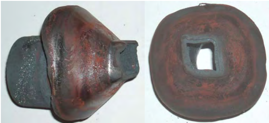
Fig. 5.7. Example of product damaged in the result of slip phenomenon ( p = 5 \text{ mm/rot.} )
