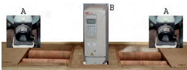
Fig. 1. Roll test bed: A - Incremental sensor of roller's revolution, B - Frequency converter
