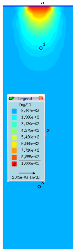
Fig. 4.68. Diagram of results of calculation of contaminant intensity in soil column
