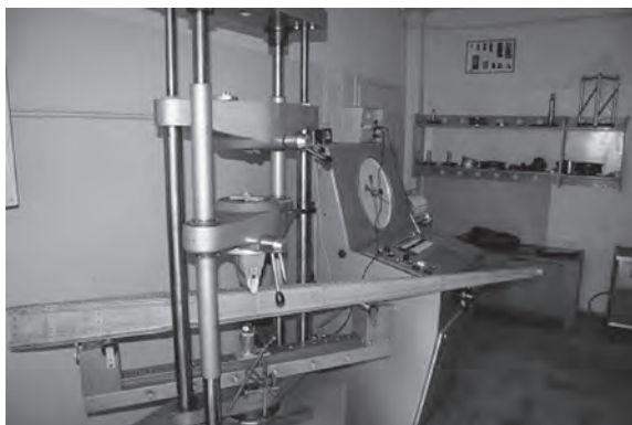
Fig. 3. Method of a girder mounting in the research stand
