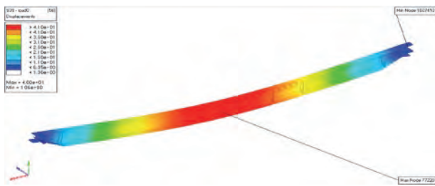
Fig. 17. Displacement cloud – “shape+size+topology” optimization
