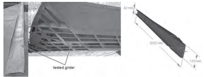
Fig. 13. The tested girder and the horizontal tail from where the girder was dismantled (left) and geometric dimensions of the girder (right)
