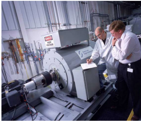
Fig. 2.14. The AMSC 5000 horse power superconducting motor under tests [68]
