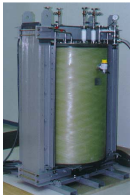
Fig. 2.15. BSCCO HTS transformer unit [83]
