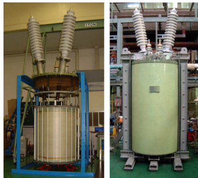
Fig. 2.16. The 2 MVA HTS transformer before (left) and after (right) the assembly [15]
