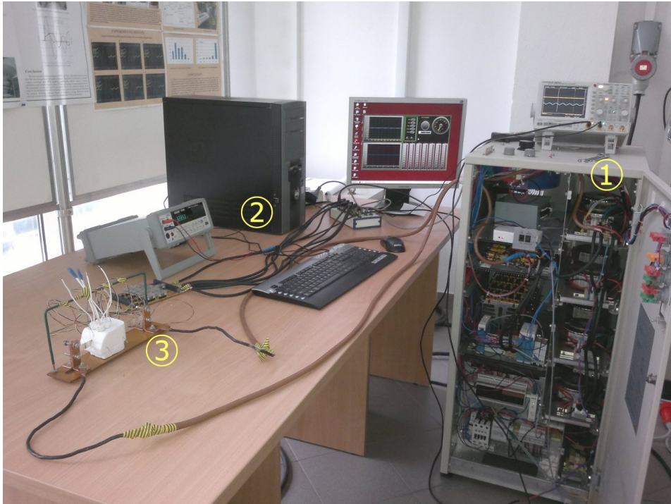
Fig. 4.2. The test stand for measuring the parameters of tape in transient states: 1 – computer controlled supplying system, 2 – data acquisition stand, 3 – HTS 2G tape with quench system
