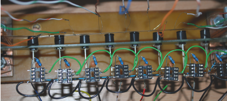
Fig. 4.62. HTS 2G tape and SFH203FA photodiodes in casings set in for measuring
