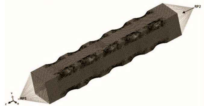
Fig. 7. The ABAQUS model of the column with distorted FEA mesh, applied load and boundary conditions
