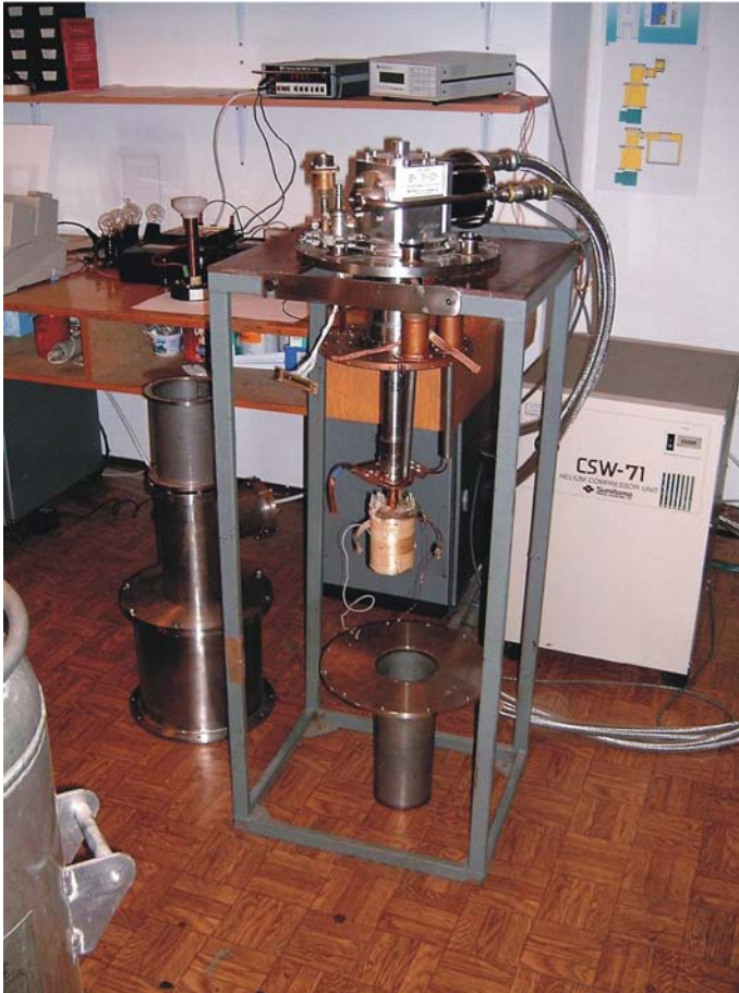
Superconducting electromagnets cooled by cryocooler
