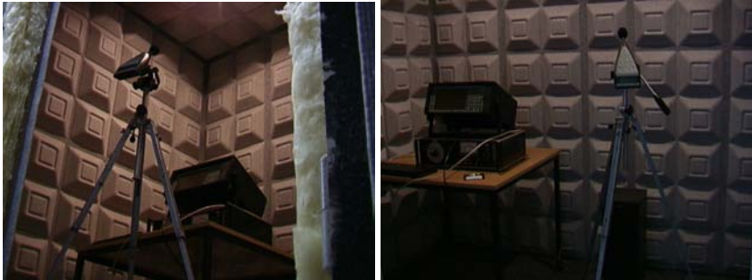
Electromagnetic and acoustic shielded chamber (size: 2,5 m x 2,6 m x 2,0 m) Analyser Bruel & Kjaer 2144, sound measuring meter FALCON 2669, disturbance measuring meter EM
