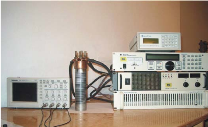
Test stand for investigation of resistive Superconducting Fault Current Limiter
