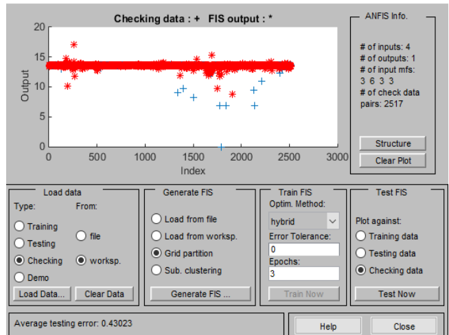
Fig. 7. The results of accuracy evaluation of the neuro-fuzzy network for air consumption of the RS's ventilation system on the test dataset
