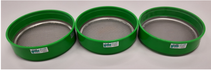
Figure 7.2. Sieves with mesh diameters: 2.24 mm (left), 1.25 mm (middle), 0.4 mm (right). Source: own elaboration
