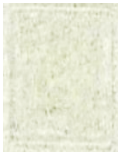
Figure 9.7. Photograph of the a-C:H film on fused silica substrate. Before doping, the film is transparent due to the high optical gap. Source: own elaboration
