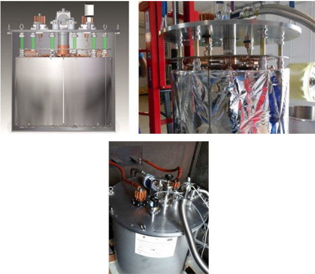
Figure 6.18. Contact-cooled superconducting fault current limiter (Electrotechnical Institute, University of Zielona Góra and Frako-Term). Source: own elaboration
