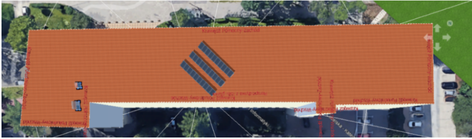
Figure 11.27. Visualisation of a PV installation with modules facing south-west on the roof of the Faculty of Electrical Engineering and Computer Science of LUT. Source: own elaboration
