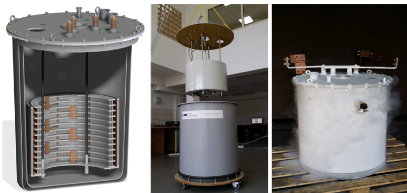
Figure 6.16. Inductive superconducting short-circuit current limiter rated at 15 kV/140 A. Source: own elaboration
