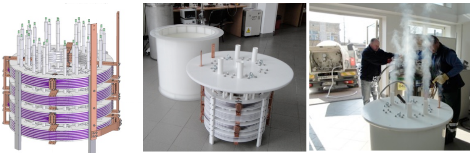
Figure 6.14. Inductive superconducting fault current limiter rated at 6.9 kV/600 A. Source: own elaboration
