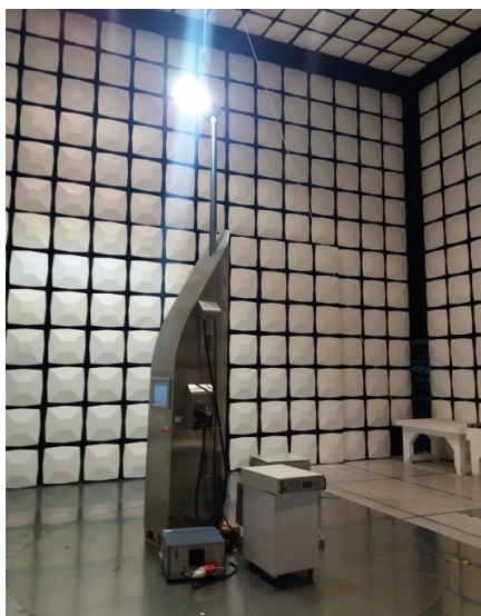
Figure 8.8. The PLUGinEV charging station, photo in the screen chamber. Source: own elaboration
