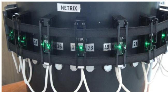
Fig. 1. UST active probes on the measuring tank
