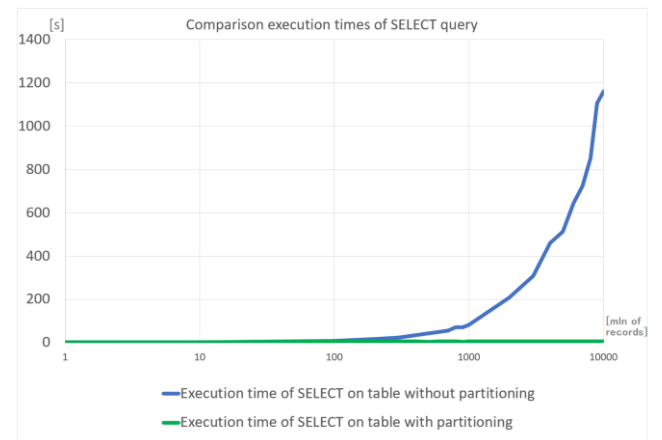
Fig. 3. Execution times of SELECT query on a table with and without partitioning, on a logarithmic scale
