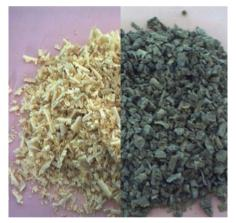
Fig. 4. Fine sawdust before (left) and after (right) drenching it in a protective mixture made of cement and water. *Source:* [3]
