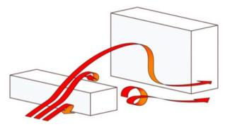
Fig. 5. The downwash vortex effect. Adapted from [4]
