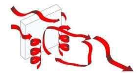
Fig. 2. Wind flow pattern on the leeward side of the building. Adapted from [4]
