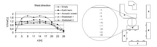
Fig. 10. Distribution of V/V<sub>o</sub> ratio in the corridor between buildings 2 and 4 for different windbreaks and west wind direction [18]
