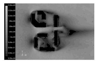
Fig. 7. Wind speed ratio for west wind direction [18]
