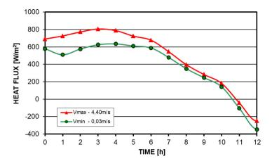
Fig.16. Heat flux for minimum and maximum wind speed from west direction [19]
