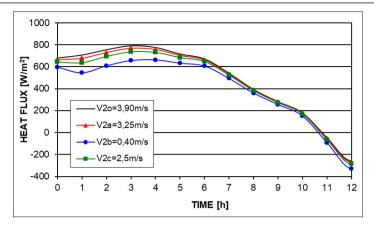
Fig. 18. Heat flux for west wind direction (Fig.15) and speeds values estimated at points 2A, 2B and 2C compared with initial value 3.90 m/s [19]
