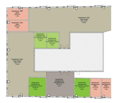
Fig. 5. Space plan with rooms' parameters transferred by Script 2 from cuboid's location. Source: own study
