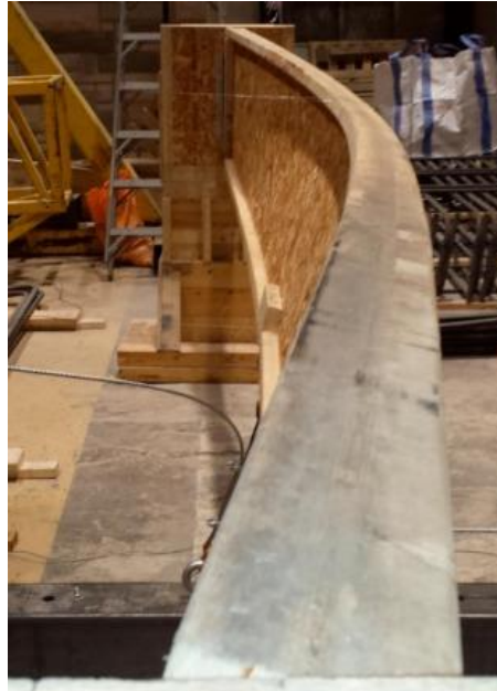
Figure 5.10. The illustration of the lateral buckling effect of the beam, showed by B. Pelletier and G. Doudak 2019
