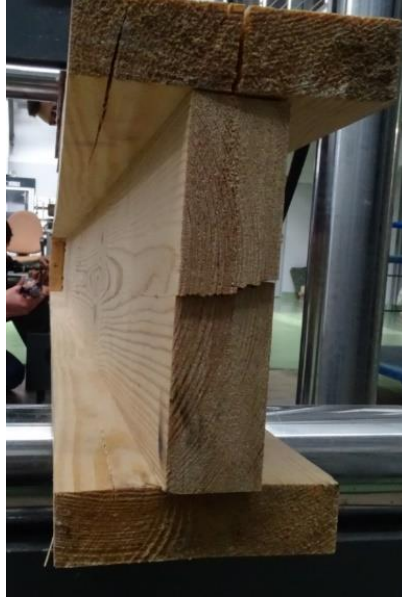
Figure 5.11. Longitudinal fracture caused by shear. Source: Author's archive
