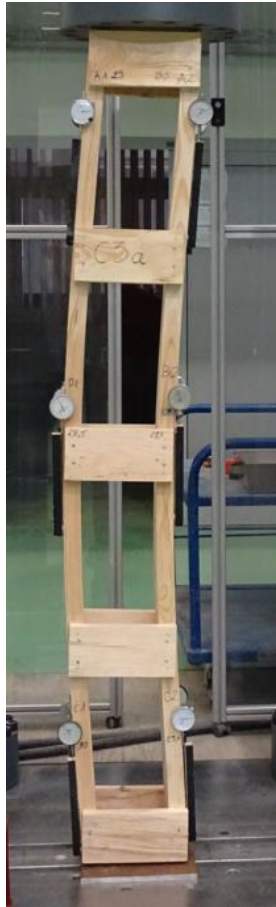
Figure 5.4. Buckling failure of a test column. Source: Author's archive
