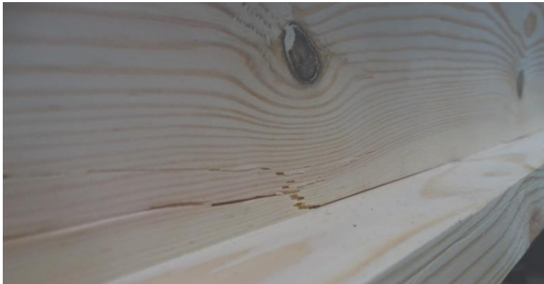
Figure 5.8. Failure of wooden fibres caused by tensile stress. Source: Author's archive
