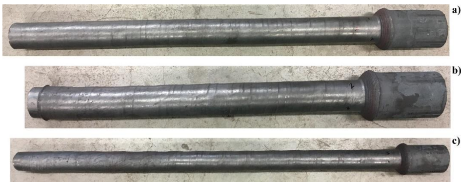
Rys. 5.61. Próbkki badawcze z widocznymi zarysami linii śrubowych: a) \alpha = 15^\circ , \theta = 7,5^\circ , V_u = 40 mm/s, \delta = 1,53 , b) \alpha = 25^\circ , \theta = 5^\circ , V_u = 40 mm/s, \delta = 1,53 , c) \alpha = 25^\circ , \theta = 7,5^\circ , V_u = 40 mm/s, \delta = 1,53
