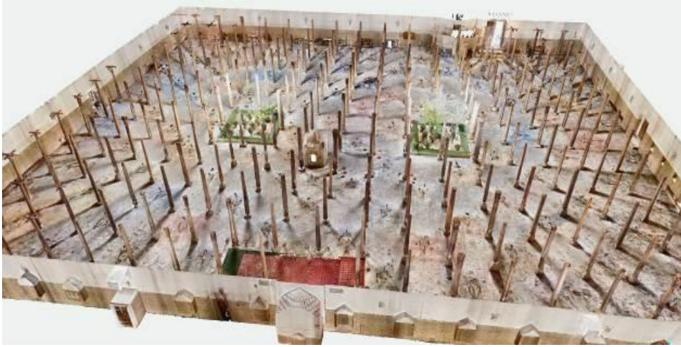
Fig. 5.19. View of the cleared point cloud after 3D scanning of the Juma Mosque. The mosque ceiling has been hidden to reveal the interior. By the authors
