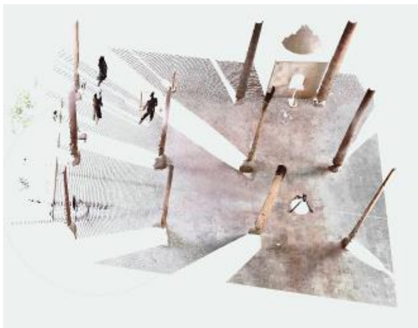
Fig. 5.18. An example of the occurrence of unwanted artefacts – people visiting the facility: (a) photo during 3D digitisation, (b) image recording from a 3D scanner. By the authors
