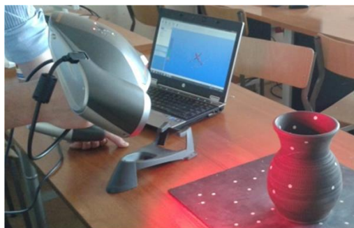
Fig. 2.2. The ZScanner ® 700: (a) general view [4], (b) the scanning process of jug [2]
