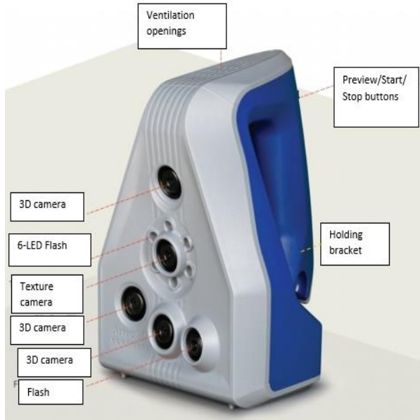
Fig. 2.5. Construction of Artec Spider scanners [11]
