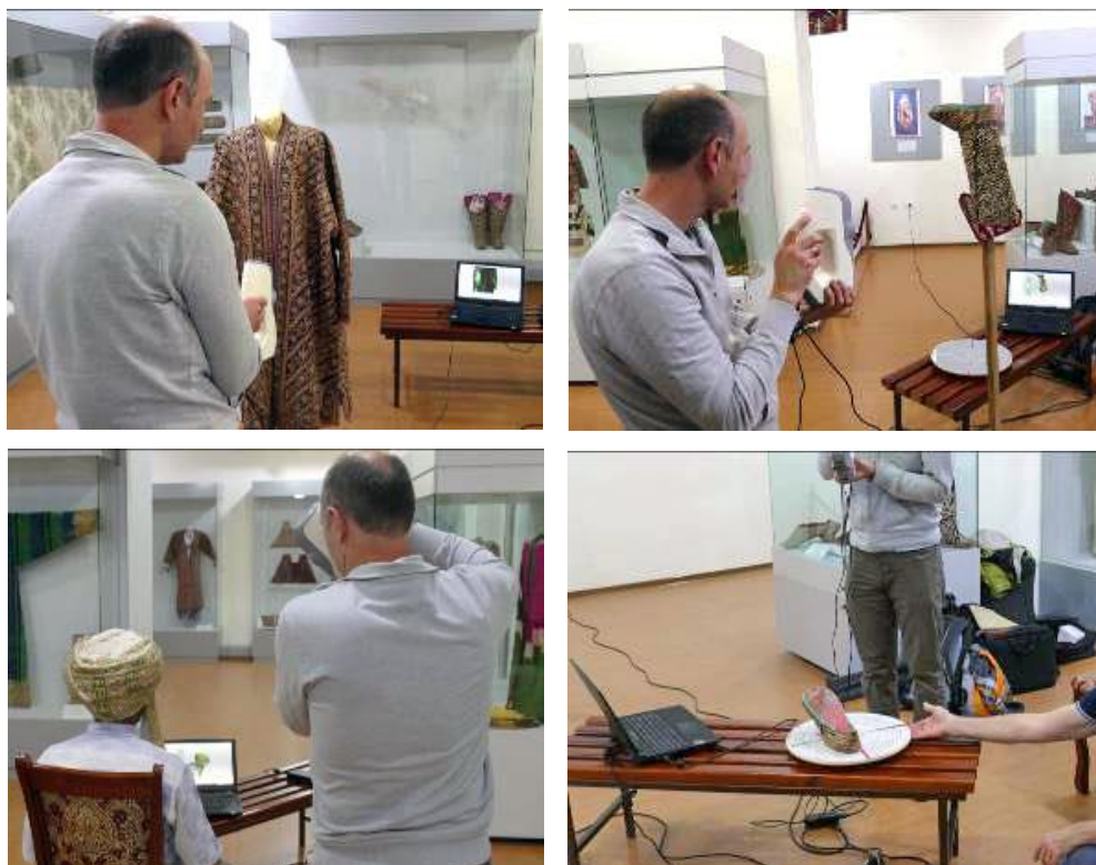
Fig. 5.62. 3D scanning of the elements of the coronation costume of the last Emir of Bukhara. By the authors
