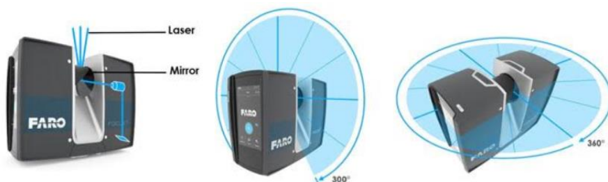
Fig. 2.3. Horizontal and vertical rotation of the laser scanner [6]
