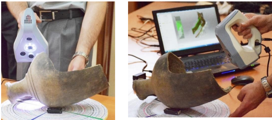
Fig. 5.20. The 3D digitisation process of the jug using the Artec Spider scanner. By the authors
