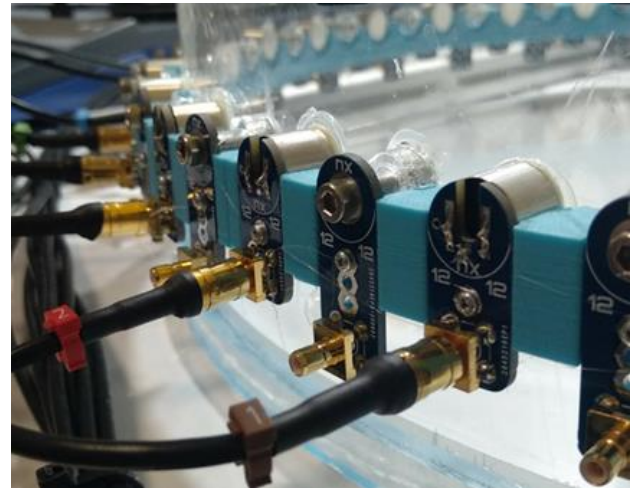
Fig. 6. Ultrasound 400 kHz transducers mounted on plexiglass tank
