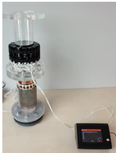
Fig. 3. Active 40 kHz probes mounted on the pipe and connected via CAN-bus
