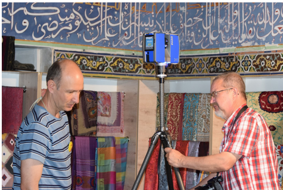
Figure 1. 3D scanning with the use of the FARO scanner, 2018, Samarkand, Uzbekistan, photo: J. Montusiewicz
