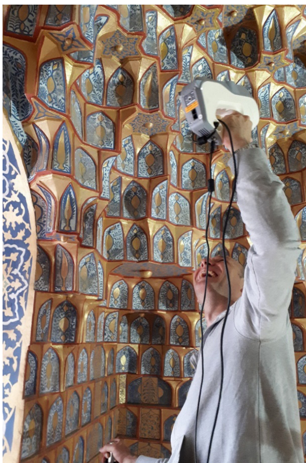
Figure 2. Scanning stalactites in the Sher-dor Madrasa by staff member of the Lublin University of Technology, photo: J. Montusiewicz
