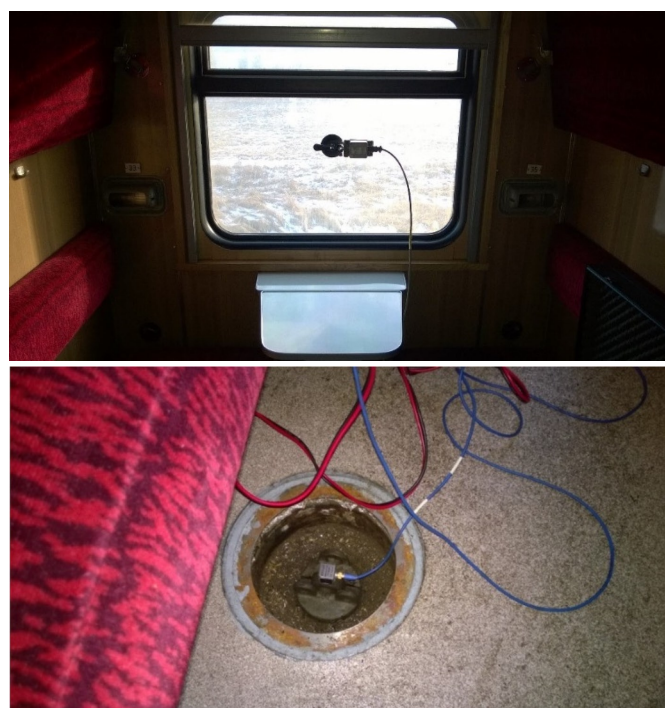
Fig. 15. Mounting of the sensors in the passenger car
