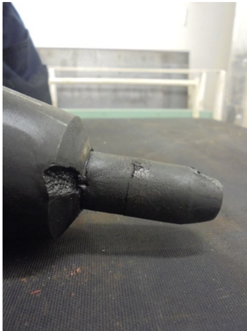
Fig. 3. High risk damage of FIV related to SECA fuel changeover, i.e. seating burnt out by combustion gas blow-by
