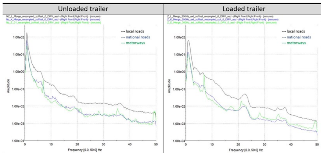
Fig. 17. Auto spectral density for estimated drive data under right front wheel for different roads
