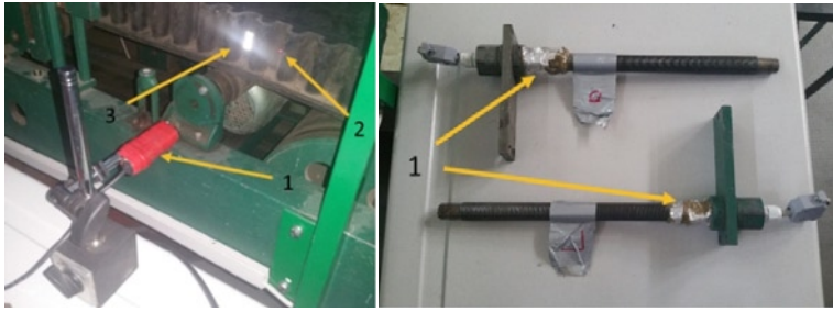
Fig. 6. Laser position sensor during work (a) and tension spindles (b)
