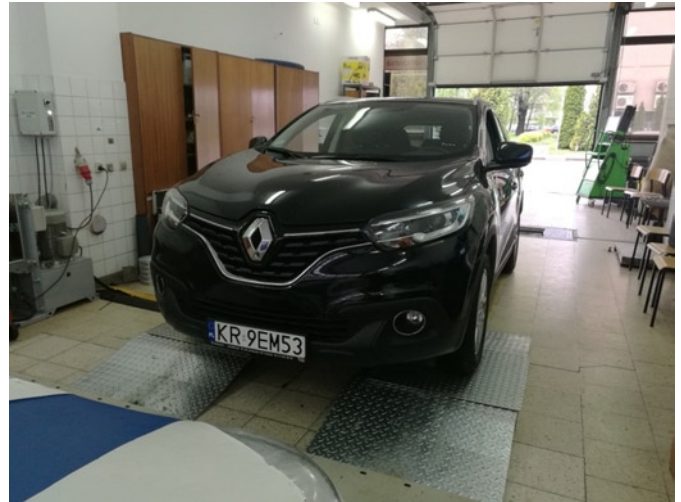
Fig. 5. Modified test stand for checking the yaw rate and lateral acceleration sensors (Unimetal Złotów) together with the test vehicle
