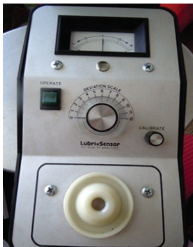
Fig. 2. Lubri Sensor applied for measurements of dielectric constant [20]
