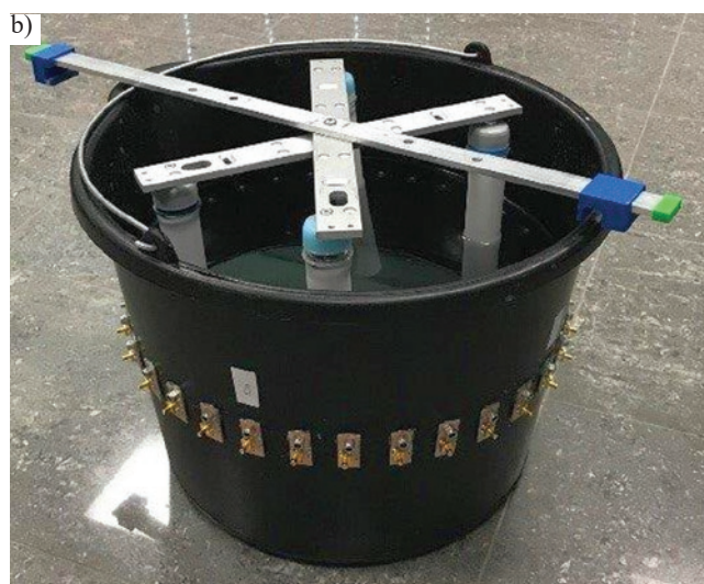
Fig. 3. The physical EIT model with the electrodes: a) schematic drawing, b) reactor with artifacts immersed in liquid electrodes
