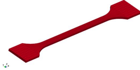
Fig. 7. Numerical model of a paddle sample
