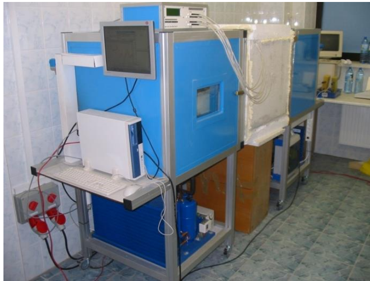
Fig. 2. Registering positions laboratory with two temperature chambers and the test material in the middle
