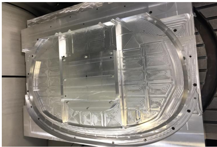
Fig. 2. The frame mounting by technological bases and additional holes during the pocket machining
