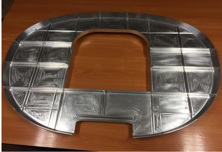
Fig. 3. The finished frame after mechanical machining (shaping)
