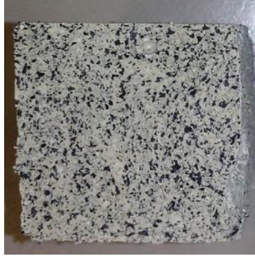
Fig. 2. Gypsum mix with 20% rubber granulate with a grain diameter of \varnothing 0.1 mm
