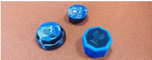
Fig. 10. The appearance of the designed beacons
