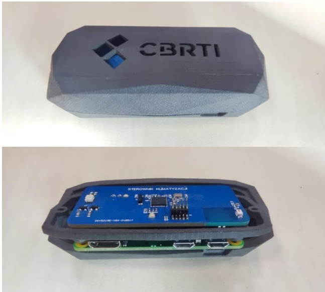
Fig. 5. The prototype of the comfort controller: the parts of the controller responsible for communication with the actuators and the single board computer managing the network communication enclosed in a single housing
