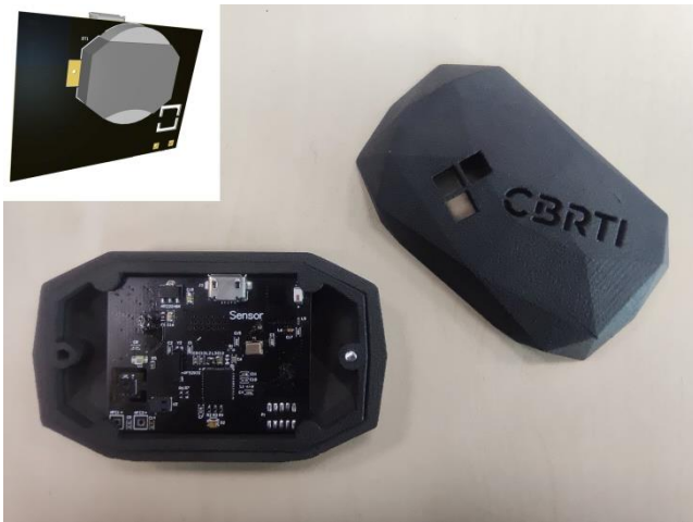
Fig. 7. Appearance of the actual environmental measuring module for indoor mounting (in the upper left corner of the drawing a 3D visualization of the PCB reverse side has been added, showing a cage for mounting a CR2032 battery with ~320 mA capacity)
