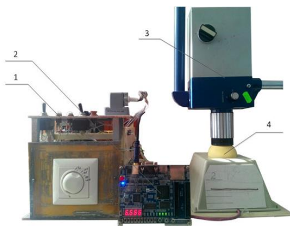
Fig. 13. GDV device for LPBO analyzing
