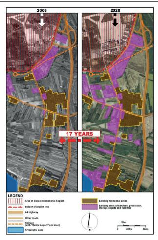
Fig. 6. Analysis of the transformation of selected elements of the functio-spatial structure in the immediate proximity of Krakow Airport in the years 2003 and 2020. *Source: own study, 2021*
