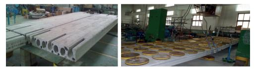
Fig. 5. Experimental investigation of hollow-core slab fragment. Source: [25]
