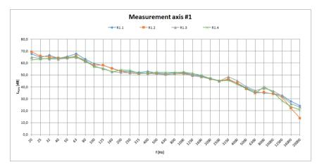
Fig. 20. Results of measurements taken at every measurement point (R1.1 - R1.4) at axis #1. Equivalent value (10 minutes) of SPL A-weighted  $L_{A, eq}$  in the function of frequency f. *Source: authors' own elaboration*
