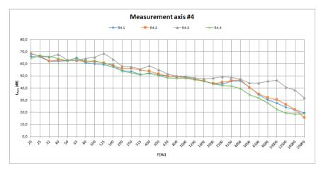
Fig. 26. Results of measurements taken at every measurement point (R4.1 – R4.4) at axis #4. Equivalent value (10 minutes) of SPL A weighted L<sub>A, eq</sub> in the function of frequency f. Source: authors' own elaboration
