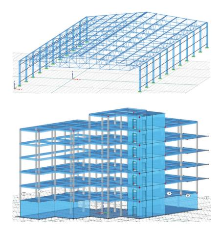
Fig. 7. View of steel and reinforced concrete structure models in RFEM obtained as result of transfer from REVIT
