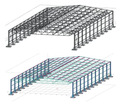
Fig. 1. View of physical models of steel structure in REVIT and TEKLA
