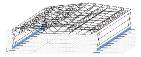
Fig. 8. View of steel structure model in RFEM after exporting it from REVIT using IFC format
