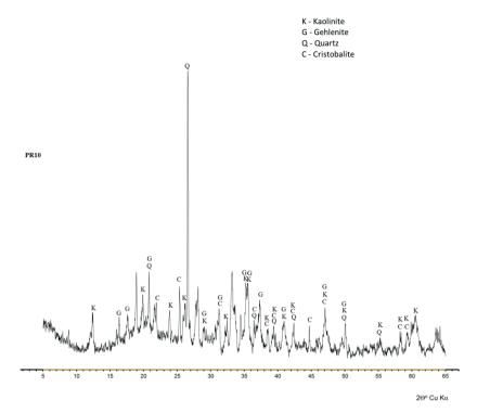
Fig. 2. Phase composition of the GD sample
