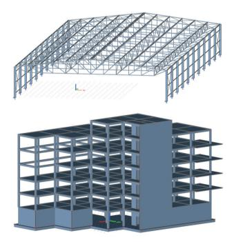
Fig. 13. View of steel and reinforced concrete structure's model in SCIA after exporting if from REVIT using plug-in
