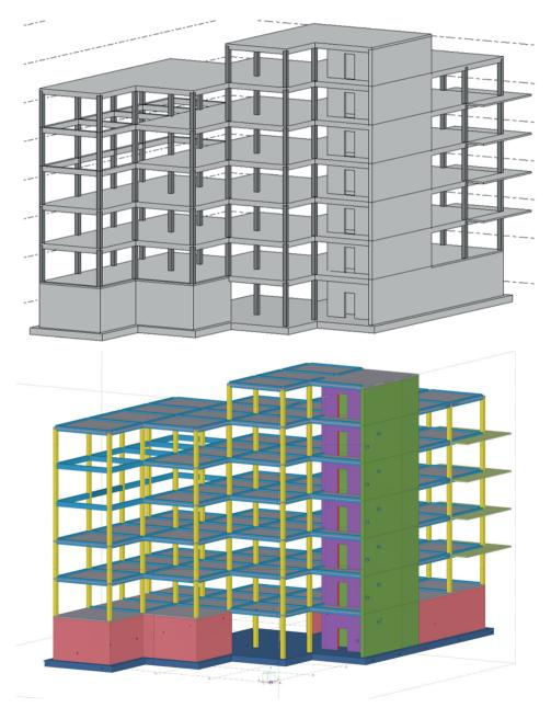
Fig. 2. View of physical models of reinforced concrete structure in REVIT and TEKLA
