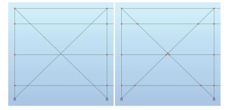
Fig. 6. Fragment of steel hall model's side elevation in ROBOT after being exported from REVIT (left) and TEKLA (right). Red dots indicate nodes created as result of data transfer
