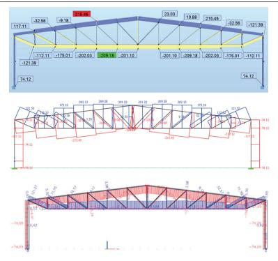
Fig. 14. Diagrams of axial forces N [kN] for selected truss module of steel structure in: ROBOT, RFEM and SCIA
