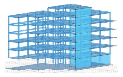
Fig. 11. View of reinforced concrete structure's model in RFEM after exporting it from TEKLA using IFC format
