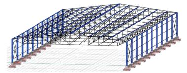
Fig. 10. View of steel structure's model in RFEM after exporting it from TEKLA using DSTV format
