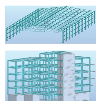
Fig. 5. View of steel and reinforced concrete structure models in ROBOT after exporting
