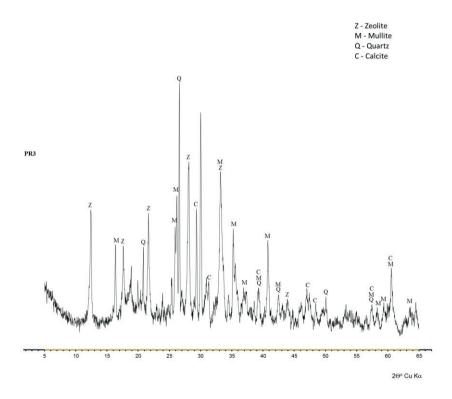
Fig. 1. Phase composition of the GZ sample
