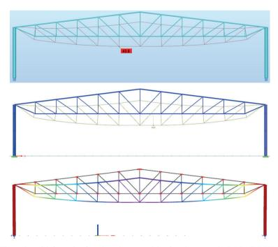
Fig. 15. Illustration of deformation for selected truss module of steel structure in: ROBOT, RFEM and SCIA
