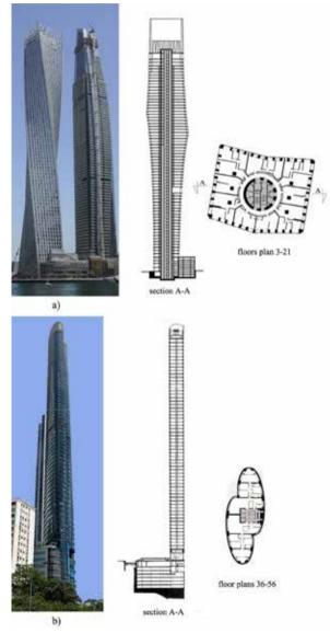
Fig. 8. Aerodynamic changing of plan geometry of residential buildings: a) Cayan Tower (Dubai, UAE);b) HighCliff (Hong Kong, China) (developed by authors)
