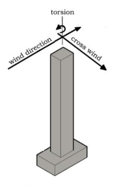
Fig. 7. Wind action on high-rise building (developed by authors based on [36])
