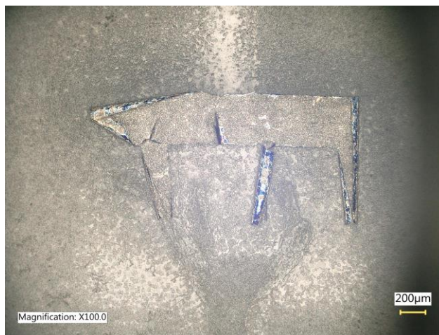
Fig. 10. Damaged nickel capacitor electrode with cells after 67 h (24 h stabilization of medium conditions and 43 h cell culture)
