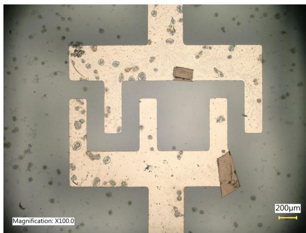
Fig. 9. Damaged nickel capacitor electrode without cells in the reference well after 67 hours (24 h stabilization of medium conditions and 43 h cell culture)
