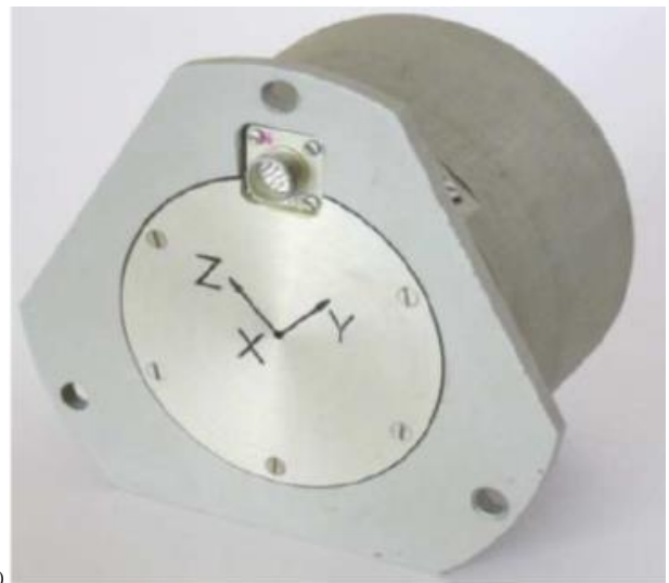
Fig. 2. Implementation of inertial orientation microsystems based on Kalman filter: for the MR control circuit (a) and for the backup orientation system (b)
