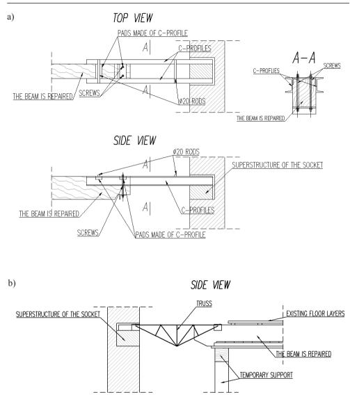
Fig. 3. Replacement of support zones of wooden beams for steel elements: a) truss, b) profiles [4]
