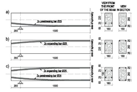
Fig. 9. The course of the routes of prestressed and expanded bars in beams, which were examined by Cyruliński; a) prestressed beam, b) expanded beam, c) prestressed-expanded beam, [8]
