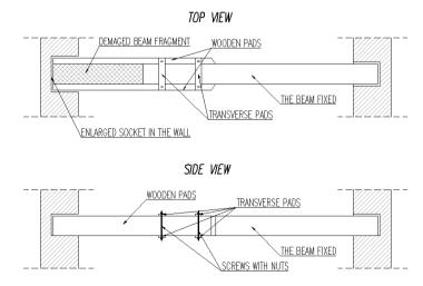
Fig. 5. Strengthening of wooden beams using wooden pads [4]
