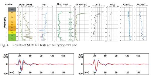
Fig. 5. Shear wave seismogram during SDMT-2 tests at a depth of 4.5 m
