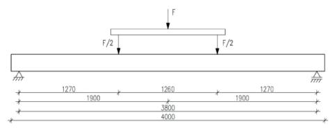
Fig. 10. Scheme of the test stand [15].
