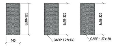
Fig. 12. Types of beams reinforced by Brol during the glued wood tests [16]
