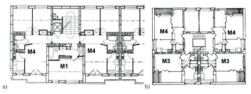
Fig. 8. Floor plans of flats: a) the Szosa Krakowska housing estate, Warsaw, 1962. b) Osiedle Młodych housing estate in Warsaw, 1962. Source: own study based on [25]
