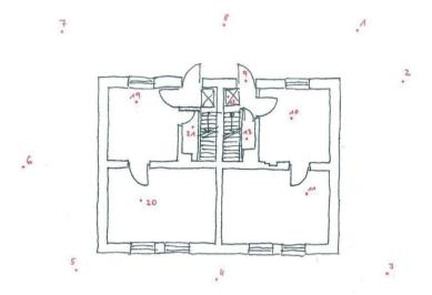
Fig. 5. An example of a manual layout sketch with marked points
