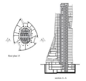
Fig. 24. Mode Gakuen Spiral Towers: floor plan and section, developed by authors [17]
