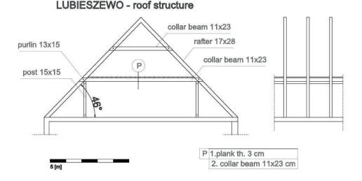
Fig. 21. The simplified scheme of the roof structure of the arcaded house in Lubieszewo (author's study)
