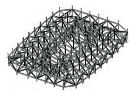
Fig. 16. Toranomon Hills: Structural spatial truss on the 36th floor [12]
