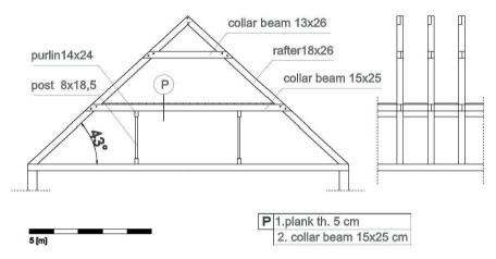
Fig. 12. The simplified scheme of the roof structure of the arcaded house in Marynowy. (author's study)
