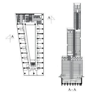
Fig. 8. Abeno Harukas: floor plan of the 53 and section, developed by authors [9]
