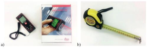
Fig. 2. Measuring instruments a) laser rangefinder b) measuring tape - photo by author
