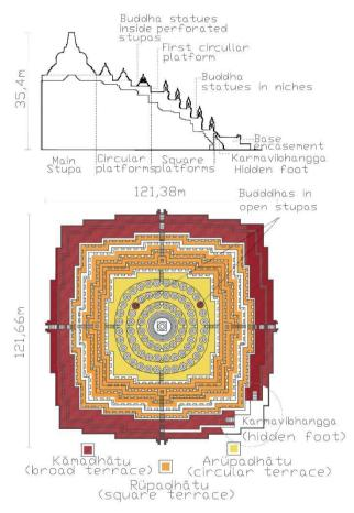
Fig. 6. Cross section and plan of the building, Borobudur, Indonesia; based on: Gunawan artapranata, https://commons.Wikimedia.org/wiki/File: Borobudur\_Cross\_Section\_en.svg, accessed 14.10.2018
