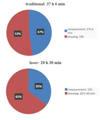
Fig. 7. Percentage comparison of measurement duration with drawing duration - compilation by the author
