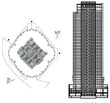
section A-A Fig. 18. Roppongi Hills Mori Tower: floor plan and section, developed by authors [13]
