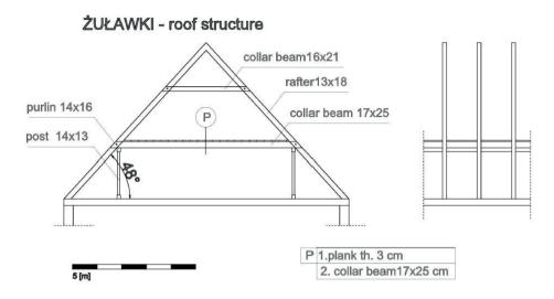
Fig. 22. The simplified scheme of the roof structure of the arcaded house in Żuławki. (author's study)
