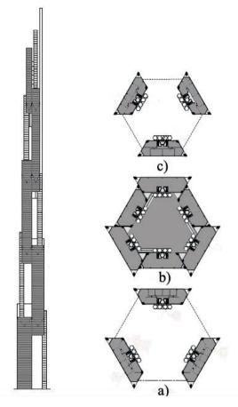
Fig. 4. Sky Mile Tower: floor plans (a) 1-35 floors; b ) 36-40 floors; c) 41-75 floors) and section, developed by authors [3]
