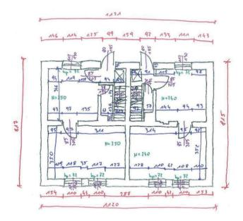
Fig. 4. An example of a manual sketch layout with dimensions
