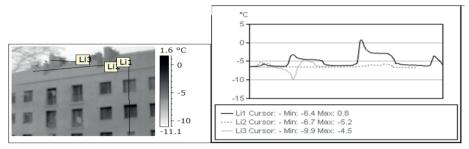
Fig. 4. Southern Poland 2012, a building made in the traditional technology after insulation. Thermogram and the analysis of a fragment of longitudinal elevation (window, woodwork, chimneys) – description in the text
