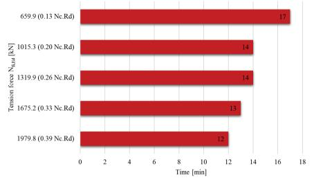
After the evaluation of the critical temperature of the joint, the fire resistance time was calculated (see Fig. 6). A standard fire was used to heat up the joint.
