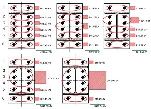
Fig. 3. Resistance of the joint at normal temperature
