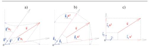
Fig 1. Base vectors as well as the contravariant and covariant vectors' components in two dimensions a) covariant vector components b) contravariant vector components c) Cartesian coordinate system
