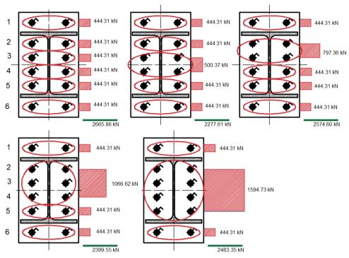
Fig. 4. Resistance of the joint at 500 °C
