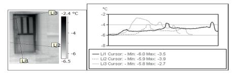
Fig. 10. Southern Poland 2012, a building made in the traditional technology after insulation. Thermogram and an analysis of the entrance door – description in the text
