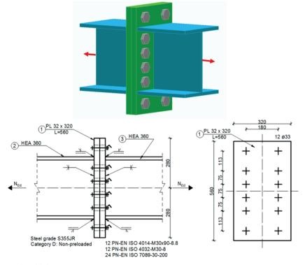
Fig. 2. Analysed joint
