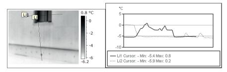
Fig. 7. Southern Poland 2012 a building made in a traditional technology after insulation. Thermogram and the analysis of a window in a gable wall and the area of the ground course – description in the text.
