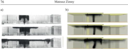
Simulation of smoke spreading in a building - comparison of methods, a) analog simulation with salt water (inverted image), b) CFD computer simulation, Source: Own study based on [19]
