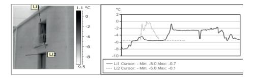
Fig 2. Southern Poland 2012, a building made in the traditional technology after insulation. Thermogram and the analysis of a fragment of the gamble wall with a portfenetre – description in the text
