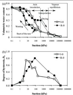
Fig. 1 Comparison of water retention curves (a) and hysteresis level (b) for intact loess and reconsolidated loess.
