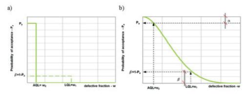
Fig. 2. Diagram of: a) an ideal OC-line and b) a real OC-line
