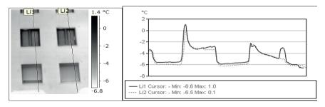
Fig. 6. Southern Poland 2012, a building made in the traditional technology after insulation. Thermogram and the analysis of window woodwork in a longitudinal wall-description in the text'
