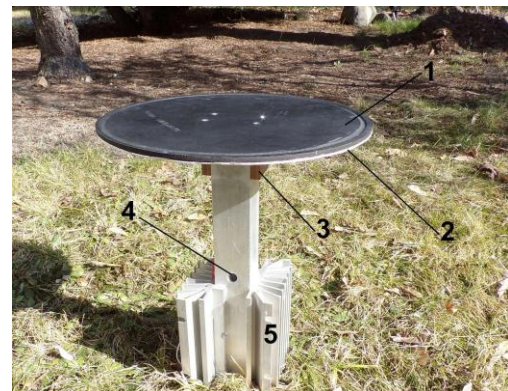
Fig. 2. Thermoelectric device prototype without the cover glass and the buoyancy tube. 1 – circular absorber plane, 2 – styrofoam layer (thermal isolation), 3 – bakelite connectors, 4 – flat aluminum profile and the upper hole of the internal channel, 5 – radiators
