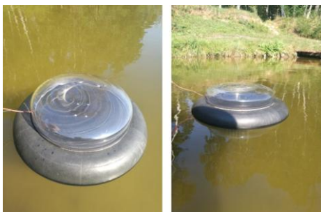
Fig. 3. Thermoelectric device prototype at the beginning testes while floating on water surface
