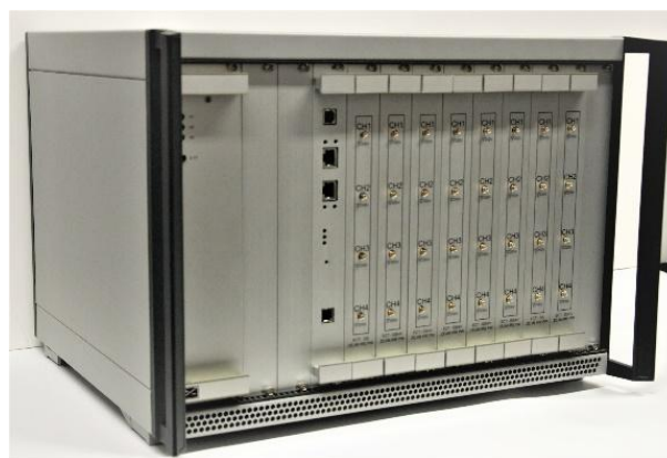
Fig. 1. EVT4 data acquisition system for ECT
