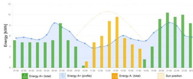
Fig. 10. Graph of energy consumed (A+) and donated (A-) in Sector 5 LSTP on a weekday – June 13, 2019
