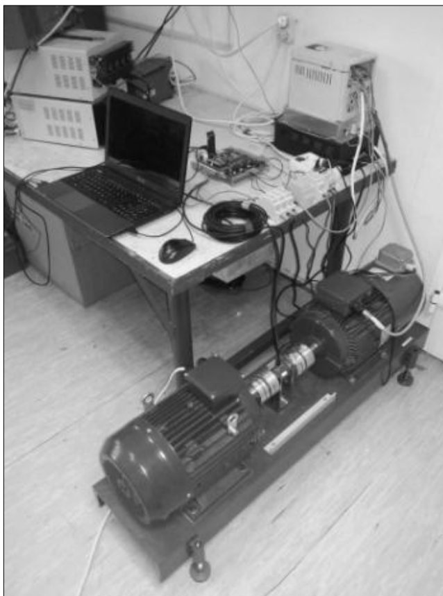
Fig. 6. Laboratory stand for small wind turbine simulation
