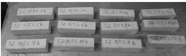
Fig. 3. Beam samples for bending strength tests
