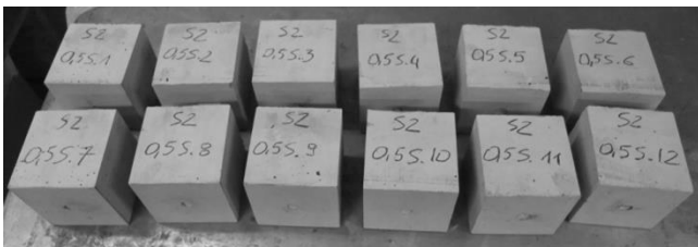
Fig. 2. Cubic samples for compressive strength tests
